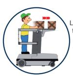
Loading platform at maximum height corresponds to the column. It is very easy to place even heavy packages using the column as the setting base and letting it slide into the material tray
